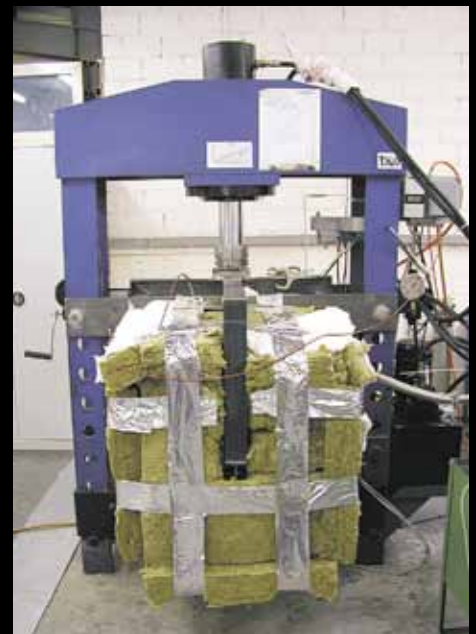
Fatigue life test under vacuum and temperature 150° C for IPP Wendelstein 7-X
